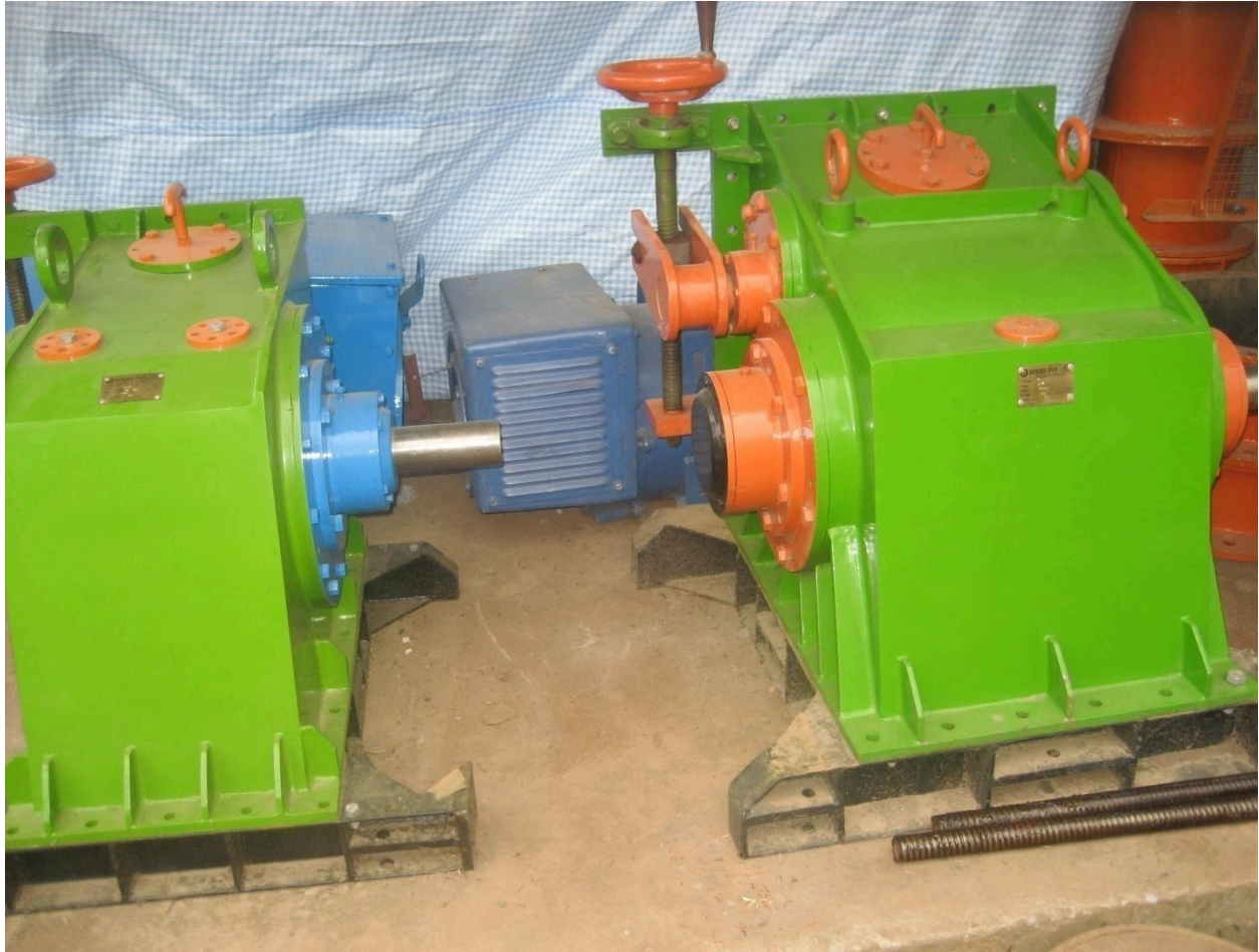
Cross Flow Turbine inside the workshop store house
