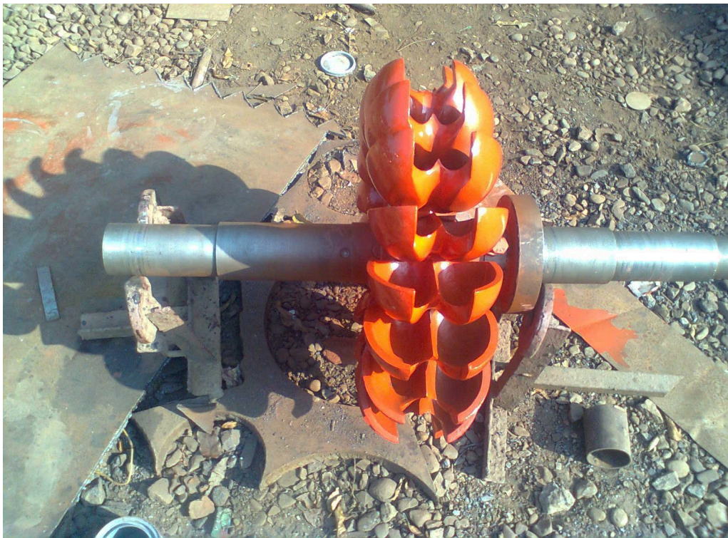
Runner of Pelton Turbine – 63 KW
